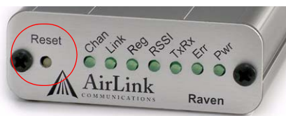
FIGURE 5. Bouton Reset du modem Raven-E
